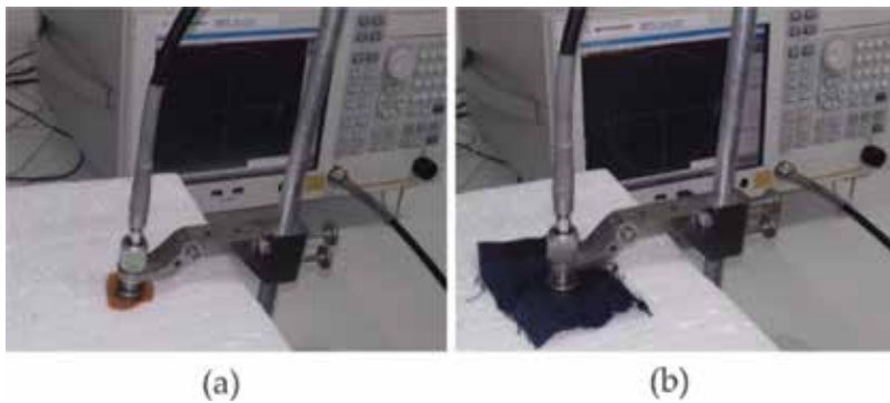
Figure 2. Electrical characterization measurement setup: (a) polyamide; and (b) denim.
