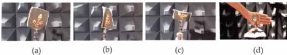
Figure 12. Measurement of prototype of the wearable textile antenna bio-inspired in Bidens pilosa plant shape: (a) free space; (b) creased; (c) bended; (d) on the hand.
