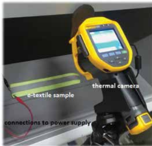
Figure 10. Testing set up to measure surface temperature.
