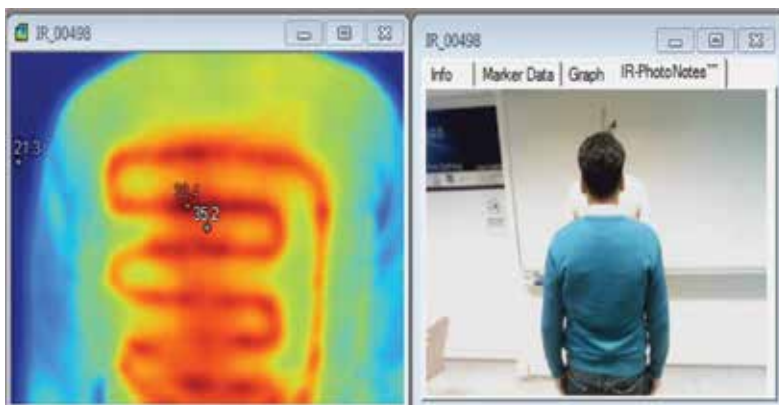
Figure 22. 10 min after wearing the heating vest (Back surface temperature on the top clothing of wearer: 38.4°C, ambient temperature: 21°C).
