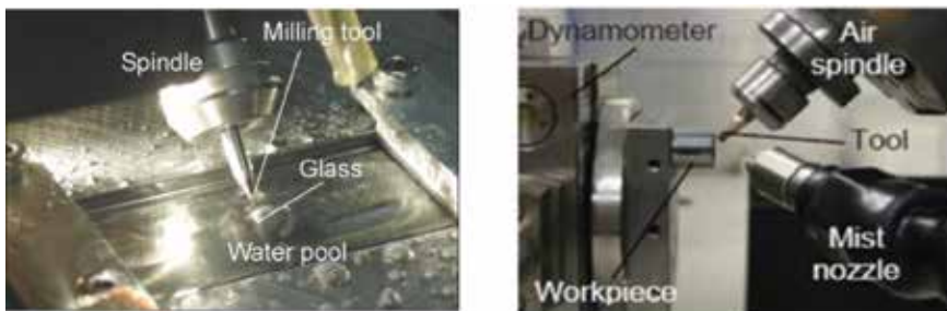
Figure 3. Schematic illustration of milling and turning processes.
