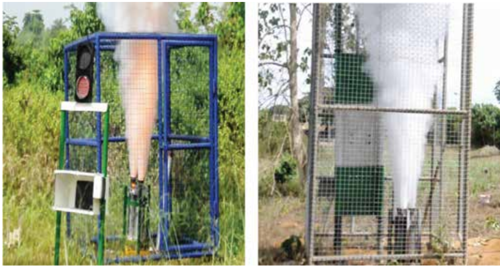
Figure 8. Static test rigs with tri-cluster rocket motors.
