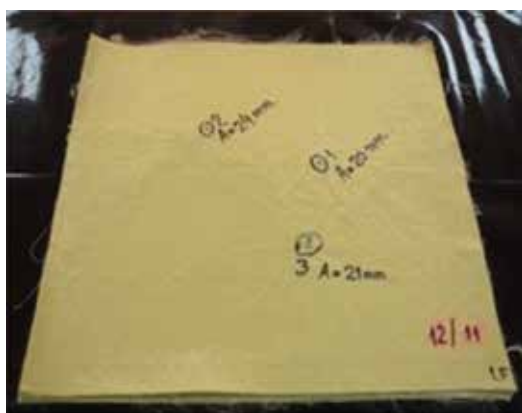
Figure 6. Tested panel made of 12 layers of LFT SB1plus.
