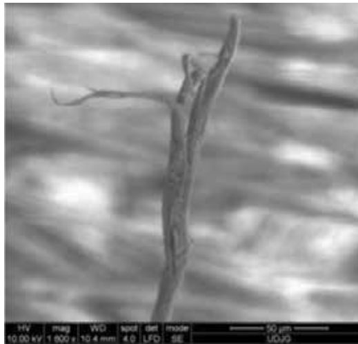
Figure 13. A fiber broken on the back of the last layer (the 12th layer).
