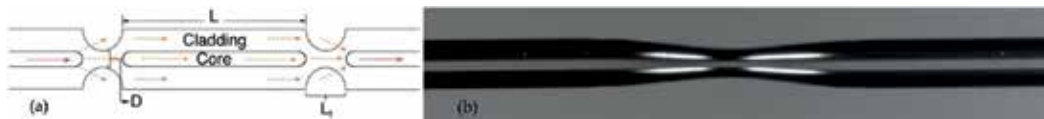
Figure 6. (a) Schematic diagram of an abrupt tapered fiber In-Line MZI; (b) microscopic image of the fabricated abrupt tapered fiber.
