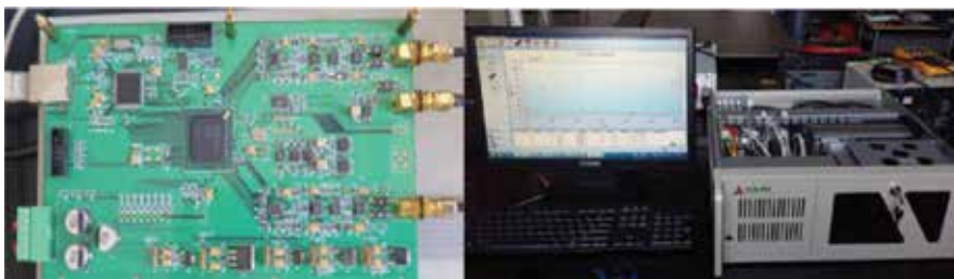
Figure 2. Developed DAQ card and DTS system for temperature measurement.
