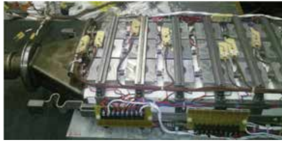
Figure 3. Skutterudite based TEG system with a rated power output of 330 W for FTP city drive cycle.
