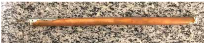
Figure 5. Assembled heat pipe.
