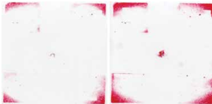
Figure 7. Pressure films for (a) four screws, 1 Nm (b) five screws, 2 Nm.
