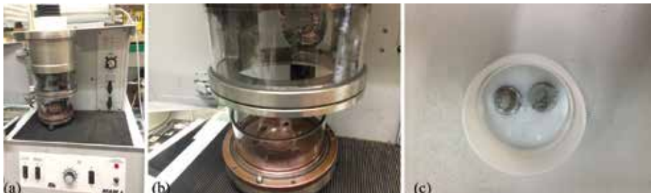
Figure 1. (a) Images of the mini arc furnace and (b) its water-cooled copper crucible, for synthesis of SnSe alloys materials. Pellets of powders of starting material are molten and then quenched in this crucible. (c) Typical disks of as-grown and then pressed intermetallic alloys.
