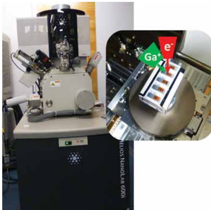
Figure 6. Fiber-milling system by focused ion beam (FIB).
