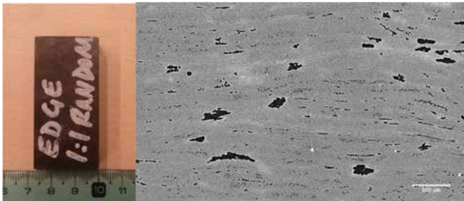
Figure 7. Left: a micro-CT sample prepared from the center coupon of COSB. Right: a 2-D micro-CT image of cured COSB sample (resolution: 2.5 \mu\text{m}/\text{px} ). Deformed prepreg strands and their curvature were observed. Morphology of the voids was also presented.
