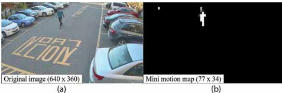
Figure 3. Mini motion map for reducing the unnecessary computation in the HOG-based human detector: (a) original image with a size of 640 \times 360 and (b) mini motion map with a size of 77 \times 34 , which was calculated from the GMM-based motion detection.
