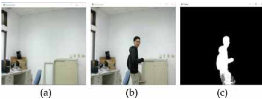
Figure 3. Foreground pixels representing the moving objects obtained by the adaptive Gaussian mixture model: (a) background, (b) moving object, and (c) foreground pixels.
