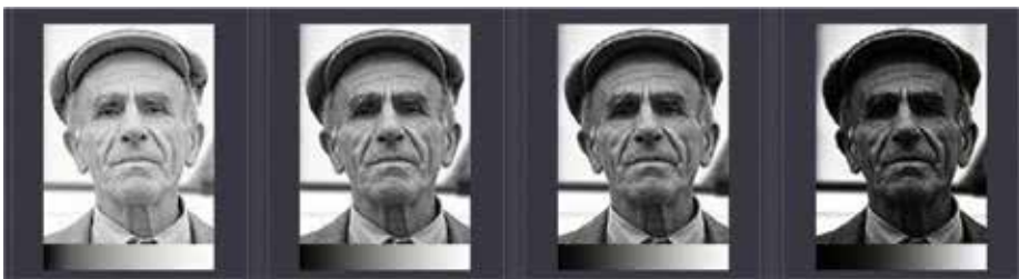
Figure 6. Face images with different gamma values. From the highest value to the lowest value (from the left to the right) ( http://www.cambridgeincolour.com/tutorials/gamma-correction.html ).
