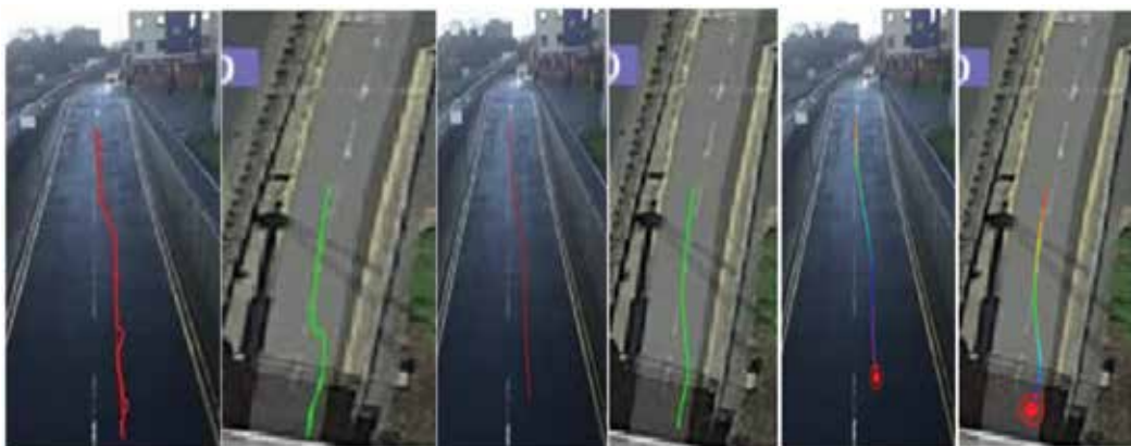
Figure 5. (a) Chaotic vehicle trajectory, (b) smooth vehicle trajectory, and (c) time stamped glyph.
