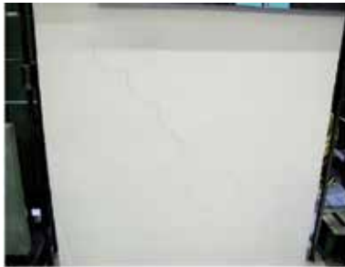
Figure 12. CS_UN: calcium-silicate brick masonry wall unstrengthened. Cracking pattern at 0.51% drift and equivalent bilinear curve.
