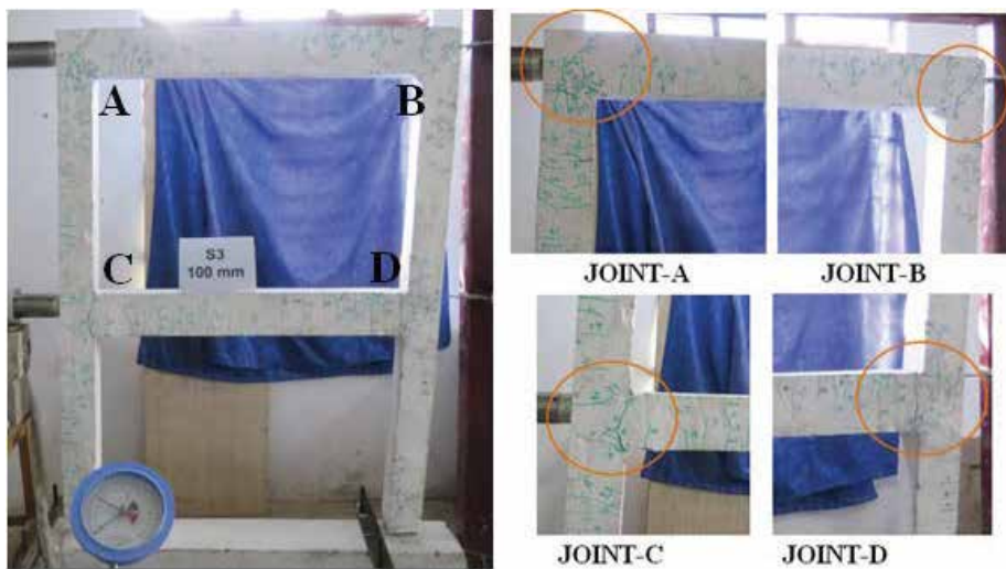
Figure 8. Failure modes of specimen S3.
