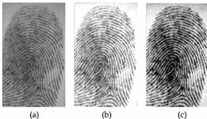
Figure 6. The original fingerprint image (a), enhanced image (b), and stretched image (c).
