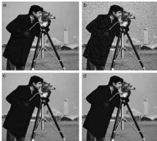
Figure 2. (a) Original image Cameraman, (b) corresponding noisy image ( PSNR = 22.1 dB), (c) denoised image after the first round of the technique proposed in [25] ( PSNR = 29.8 dB), and (d) denoised image after the second round of the proposed technique ( PSNR = 30.1 dB) [25].
