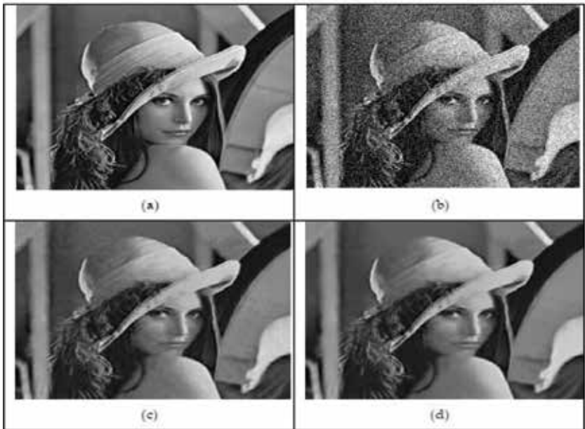
Figure 14. (a) Clean image (Lena.tif), (b) Noisy image with, (c) The denoised image by the proposed technique (the first stage) and denoised image by the proposed technique (the second stage).
