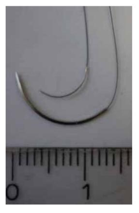
Figure 4. Onalon 6/0 microsurgical filament: fine needle, 6/0 strand.
