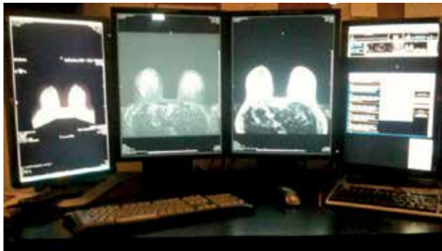
Figure 5. Image of the typical diagnostic radiology workstation displaying images of a breast MRI. Note that four flat-screen monitors are present. Methods for human machine interaction (HMI) to manipulate the images include a mouse and keyboard.
