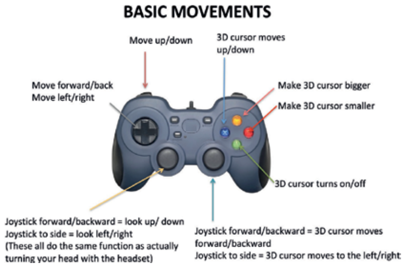
Figure 16. This figure illustrates a graphical user interface (GUI) used by D3D technologies programmed with basic movements, which are defined as a single controls input at one time.
