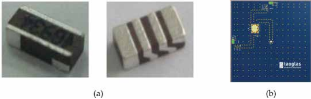
Figure 6. Chip antenna. (a) Monopole and helix by Abracon [47] and (b) Taoglass MAT.12A dual-chip antenna fed with a quadrature coupler [48].
