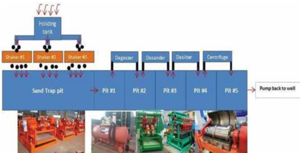
Figure 4. New design solid control system. (Note: Figures 3 and 4 is based on personal experience).
