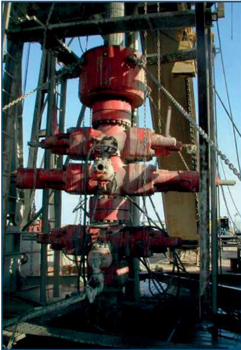
Figure 4. Typical surface BOP stack, connected to BOP control system and hydraulic power unit via flexible hoses.
