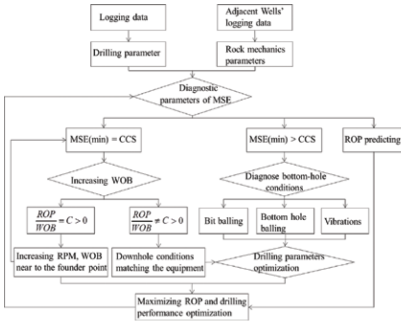
Figure 4. Flow chart of drilling performance prediction and optimization [12].
