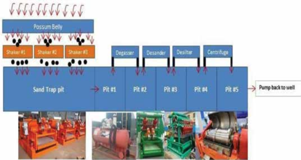
Figure 3. Old design solid control system.
