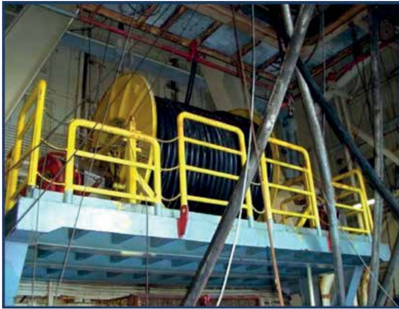
Figure 12. Typical BOP hose reel: mezzanine-deck mounted.
