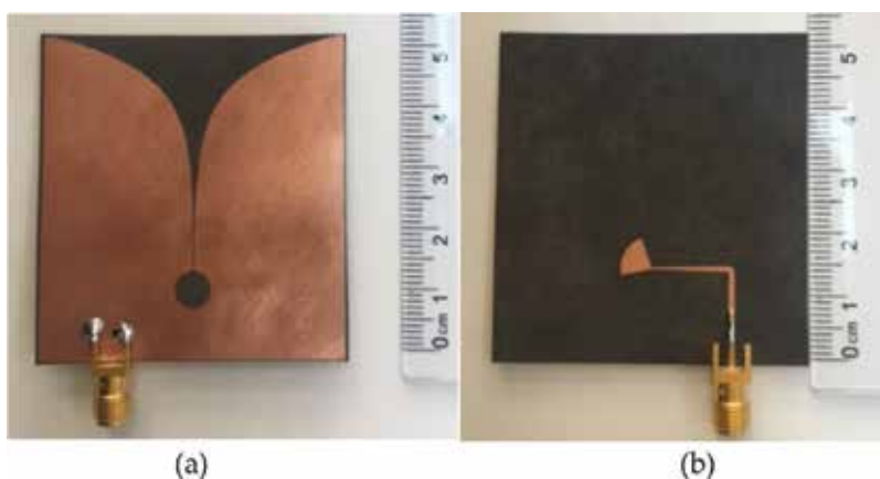
Figure 3. Fabricated Vivaldi antenna (a) top view; (b) back view.
