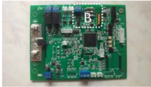
Figure 8. Architecture of EMS (symbol B is a safety device for estimating RLIB pack's insulation resistance).
