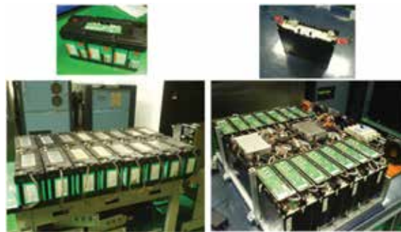
Figure 3. Reused Lithium-ion battery used in pure electric vehicles (left: \text{LiFePO}_4 , right: \text{LiMnNiCoO}_2 ).
