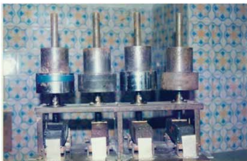
Figure 14. Vibration exciter at the moment of asphalt concrete beams testing.
