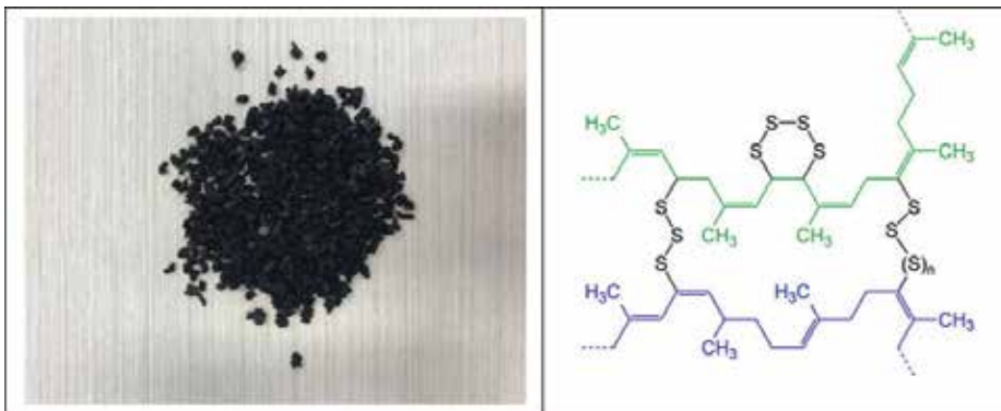
Figure 5. Analyzed material (a) crumb rubber and (b) chemical structure of rubber.
