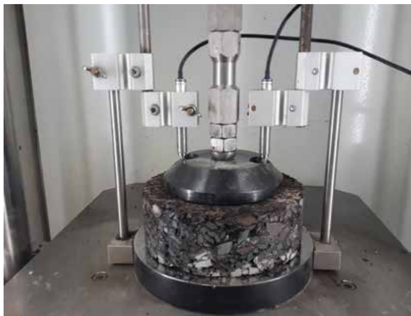
Figure 6. Creep test set-up.
