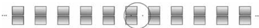
Figure 5. Scheme of the periodic field mass principle. Rest positions of the two bobs are shown (black dots). The circle in the middle represents the outline of the lower vacuum chamber through whose tunnels, shown in Figure 4 , the field systems go.
