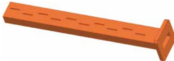
Figure 9. Geometry of conventional SWA with 15 mm slot length and 3.5 mm slot offset.
