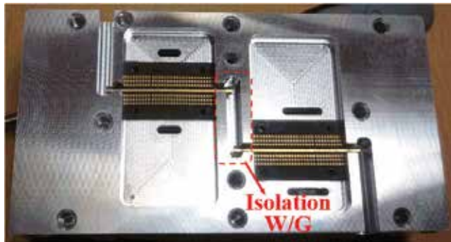
Figure 4. Fabricated transitions and assembled in the metal case.
