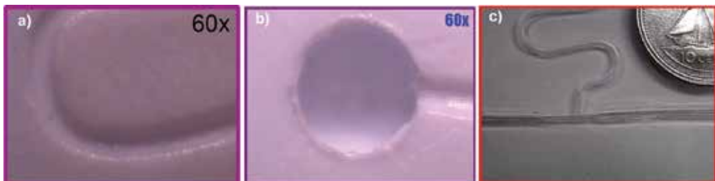
Figure 5. (a) Imprinted channel on a polymeric chip (60x magnification), (b) sample-well (60x magnification) and (c) Venturi micropump with no moving parts and no electrical power requirements fabricated by imprinting (coin included for size) [73].
