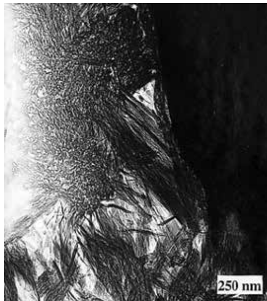
Figure 1. TEM image showing fine, dense morphology of the inner C-S-H and less dense, fibrillary morphology of the outer C-S-H formed during the hydration of C_3S [9].
