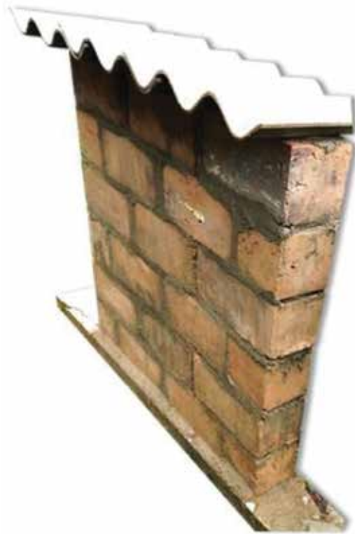
Figure 19. Fly ash geopolymerized mud concrete masonry unit wall.
