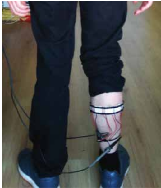
Figure 10. Thermoelectric generator on lower leg.
