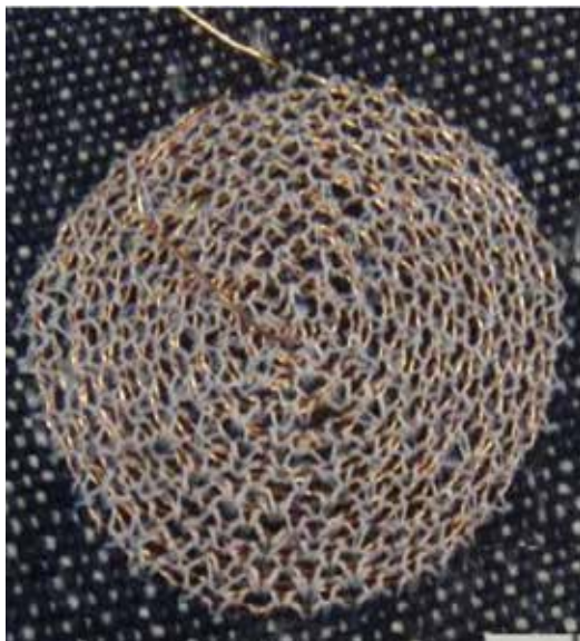
Figure 3. Copper wire sewed on a textile substrate (created in RWTH Aachen University – Institut für Textiltechnik, Aachen).
