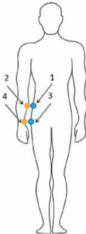
Figure 5. Positions of parts of electromagnetic harvester. 1 and 3 – Positions for flat inductors, 2 and 4 – For the permanent magnet.
