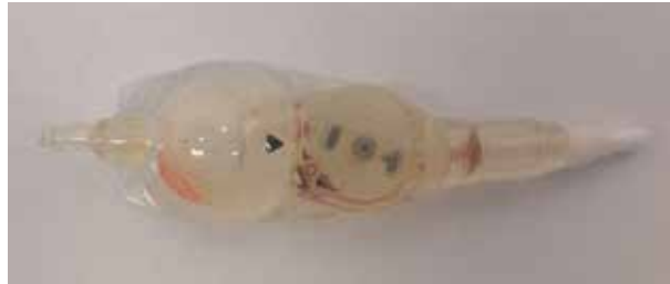
Figure 87. The blocked programmable CODMAN@CERTAS™ valve. The valve obstruction caused by blood sediment.
