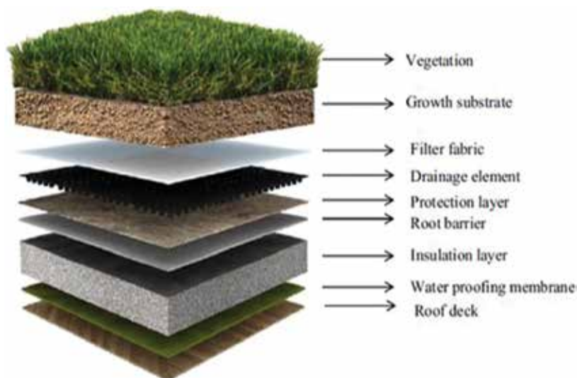
Figure 10. Schematics of different green roof components [58].
