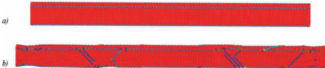
Figure 2. Red atoms: CSP \leq 21 , nonred atoms: 21 < CSP \leq 60 . [100]-orientation and s = 6a_0 . (a) \epsilon_x = 0 and (b) \epsilon_x = 0.1 .
