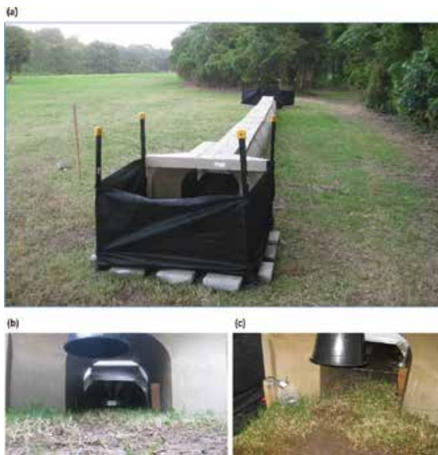
Figure 2. Experimental setup to study the tunnel-crossing behavior of amphibians. Experimental tunnel (ACO climate tunnel model KT 500) used to record amphibian-crossing movements, Photographs by Andrew Hamer (from ([52])). (a) Global view of the tunnel; (b) a view through the tunnel from the entrance arena; (c) view of the tunnel entrance with the infrared camera on the left and the temperature data logger next to the camera. The black plastic bucket is the raised acclimation chamber used for tested animals.
