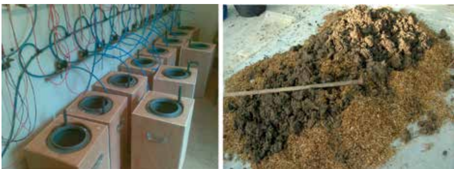
Figure 4. System of 12 composting reactors of 30 L, each one inside a wooden box for the maintenance of adiabatic conditions (left) and mixture of bulking agent with sewage sludge in 3:1 proportion in volume (right).
