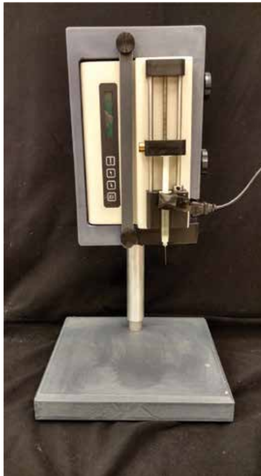
Figure 1. The KD scientific model 100 series screw-driven pressure pump with maximum force of 20 lbs is shown housed in a homemade holder attached to a vertical stand with a heavy base equipped with a 3-mL syringe and a 28G nozzle of 1" in length that was used for the experiments shown in Figures 2 and 4 ( Figure 3 has the 30G nozzle but same device).
