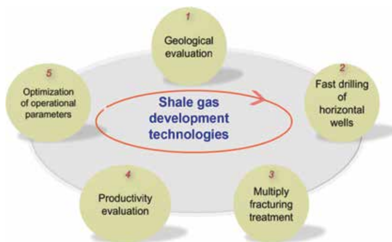
Figure 1. Schematic diagram of shale gas development technologies.
