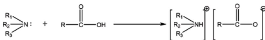
Scheme 1. Synthesis of hydroxyl amine lactate. I: (R = CH 3 , R 1 = H, R 2 = H, R 3 = HO-CH 2 -CH 2 -); II, (R = CH 3 , R 1 = H, R 2 = HO-CH 2 -CH 2 -, R 3 = HO-CH 2 -CH 2 -); and III, (R = CH 3 , R 1 = CH 3 , R 2 = CH 3 , R 3 = HO-CH 2 -CH 2 -).
