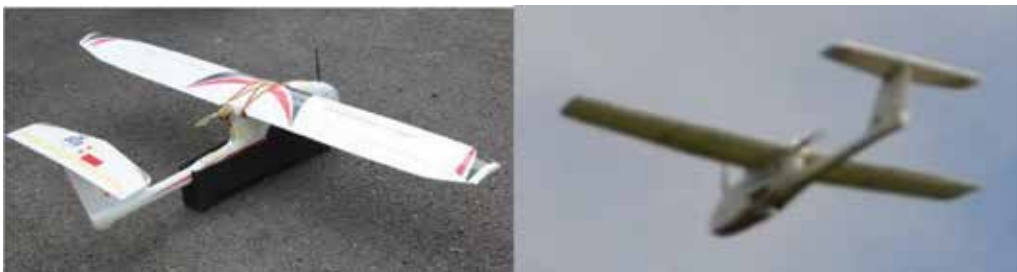
Figure 4. Left: LSU-01 final configuration; right: LSU-01 during operation with the camera bay shown under the fuselage.
