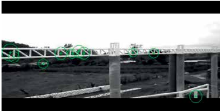
Figure 2. Result of the application of the SURF method in the image captured by the UAV.
