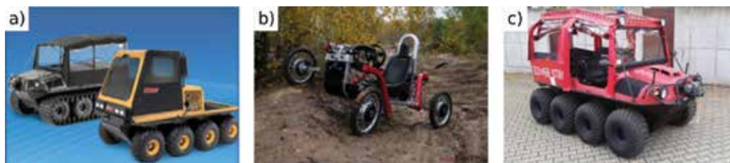
Figure 1. Example of ground units (a) adapted to driving in a complex terrain trailer pulled by Land Rover Defender 110 [3], (b) all-terrain vehicle Swincar [4] and (c) ARGO 8 × 8 amphibious vehicle in a track and wheel version [5].
