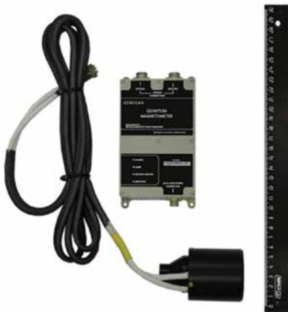
Figure 7. Rubidium vapor magnetometer (RVM).
