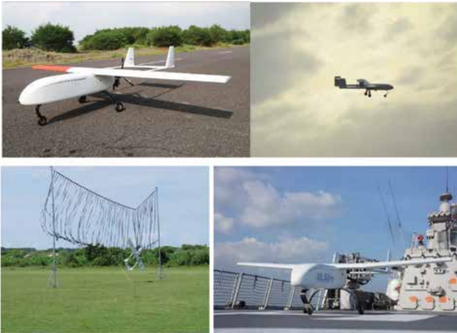
Figure 5. Top-left: LSU-02 final configuration shortly before takeoff; top-right: LSU-02 during aerial photography mission; bottom-left: landing operation with net; bottom-right: takeoff preparation from Indonesian Hasanudin class corvette warship.
