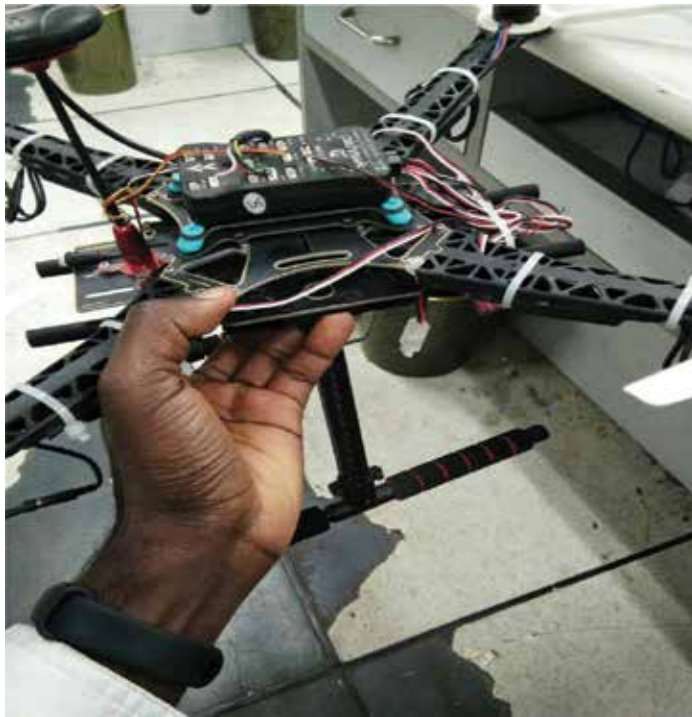
Figure 4. Smart Arduino sensor integrated drone.
