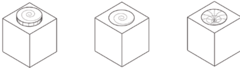
Figure 3. The control plate rising above, flush, and dropping below the top surface of the box.
