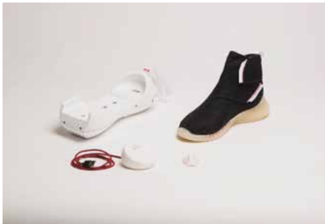
Figure 4. The physical game controller system: shoe, weighted sole, recharging dock, iMu sensors and cables.
