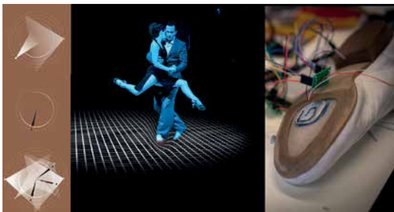
Figure 6. Exploring intentionality in tango: pressure sensors embedded in the shoes of the dancers are used to gather data and visualise pressure, force and points of contact. Photos courtesy of Murat Erdemsel.
