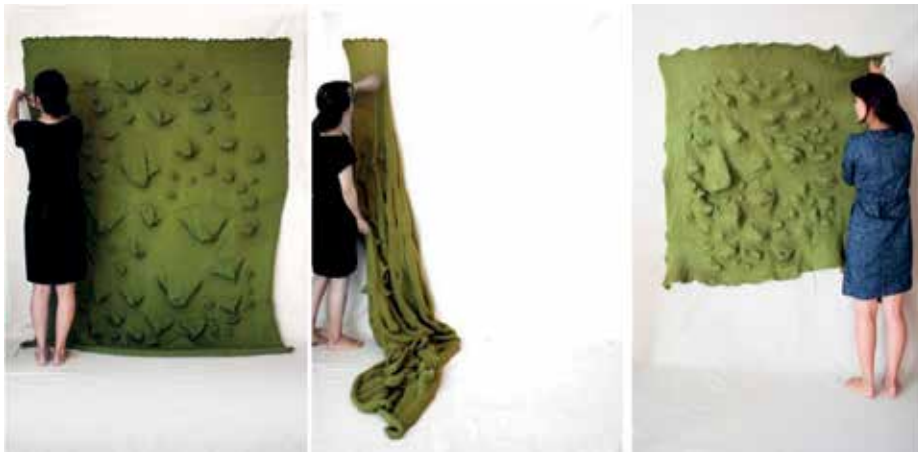
Figure 6. Felting process shrinks the woven wool textile by 30–40%. Felting transforms a woven knitted fabric into a seamless non-woven fabric.
