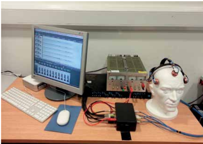
Figure 1. Prototype 5 transducer array, amplifiers, interface and DAW.
