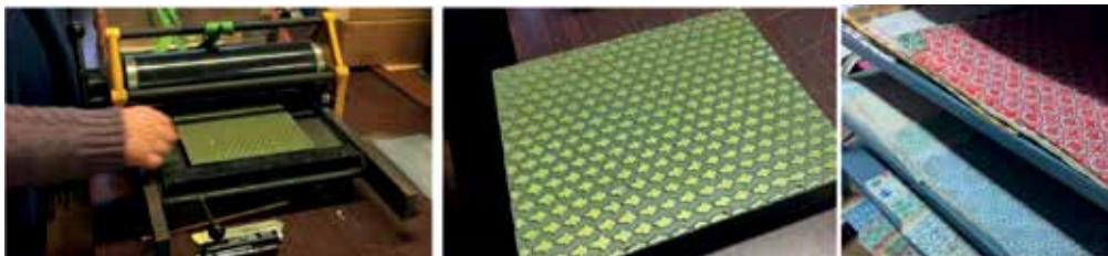
Figure 3. Using pattern blocks to print (stamp) colored patterns on paper. For complex prints with multi colors, multiple pattern blocks and inks are used during the process. A full pattern is separated into multiple blocks to allow multi-color press printing.
