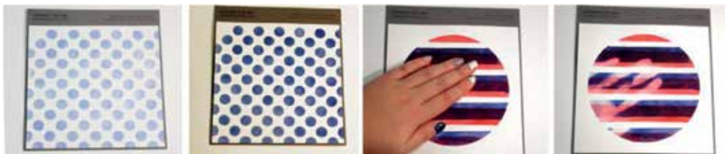
Figure 5. Using reactive pigments such as thermochromic pigments to create interactive decorative patterns on paper by painting and stenciling.
