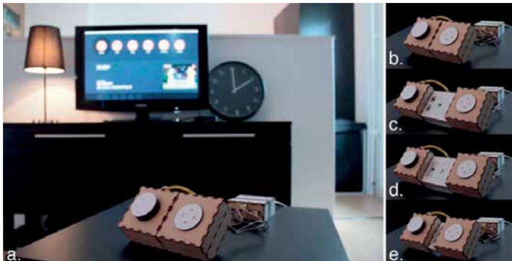
Figure 6. Adaptive remote control by Paul van Beek, 2014 (Photos courtesy of Paul van Beek). (a) The adaptive remote control in context (closed state); (b–e) Depending on the requirements of the task the remote control opens en gives context dependent controls on the slider in the middle.
