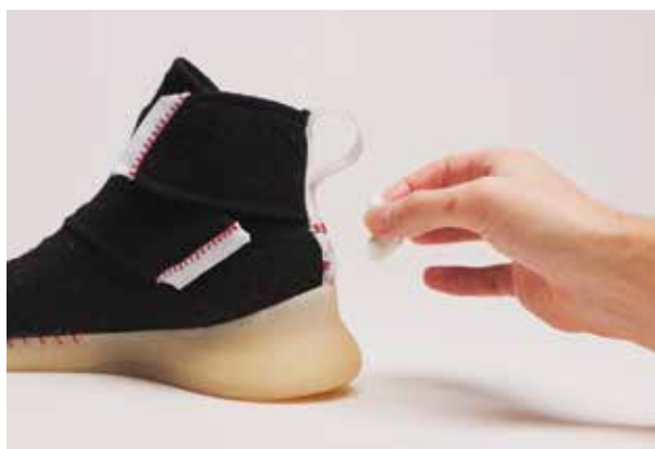
Figure 6. The iMu sensor clips into place on the back of the shoe.
