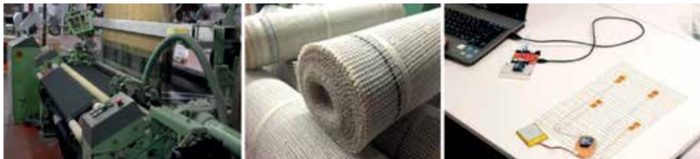
Figure 11. Left: textile mill near Florence that produces performative textiles. Middle: the woven textile inspired the potential integration of conductive fibers. Right: testing the idea of adding sensors to the conductive substrate for added interactivity and performance.
