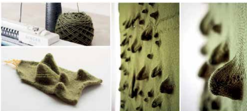
Figure 4. Knitting with two different types of yarn to create a conductive 3D structure knit. Conductive fibers are embedded in each tip of the three-dimensional forms.
