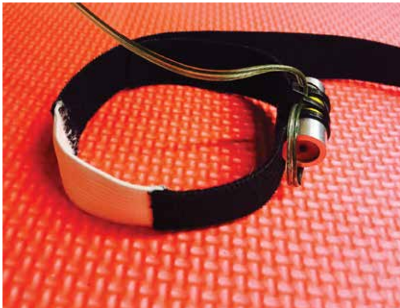
Figure 1. The vibrating band used in the study consists of a Haptuator attached to a Velcro strap.
