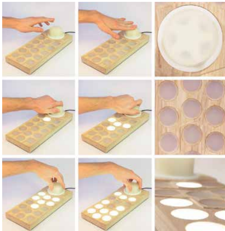
Figure 6. Design four: rotary relays. PPP 3D print, wood, Arduino microcontroller, potentiometer, and LED lights.
