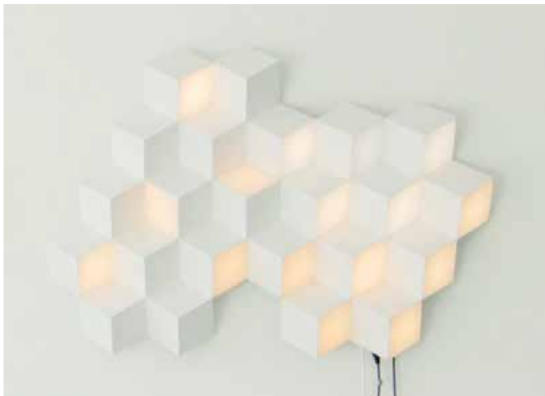
Figure 8. Integrated daylighting and artificial lighting. A close look at a section of the instrument where some surfaces are lit by daylight and some by the embedded LED. The surfaces appear in a range of lit, reflected, and shadowed showing the range of local light variations. Figure 9 shows the same section with the curtains drawn for the window, excluding the daylight.
