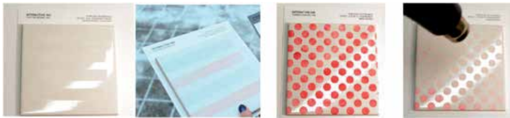
Figure 8. Thermochromic pigments were painted on ceramic surfaces: these patterns are responsive to differences in temperature, such as cold or heat.
