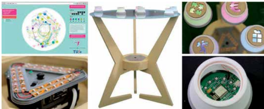
Figure 2. Elements of the [X]CP system, f.l.t.r.: real-time visualisation, table with tokens, symbols on tokens, tracking hardware and token hardware.
