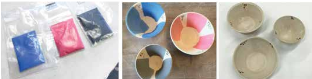
Figure 7. Thermochromic pigment powder was added to the glazing base at different concentration for glazing ceramics. However, the thermochromic glaze lost its properties under high heat during the baking process in the kiln.
