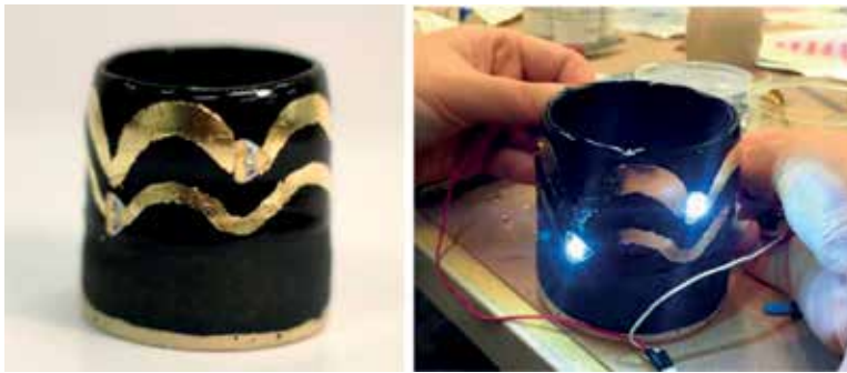
Figure 10. Testing of adding simple LED light interactivity using gilded metallic circuits.
