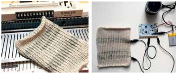
Figure 12. Conductive fibers were knitted together with regular yarn to create conductive areas for touch interactivity to generate output, such as sound in this example.
