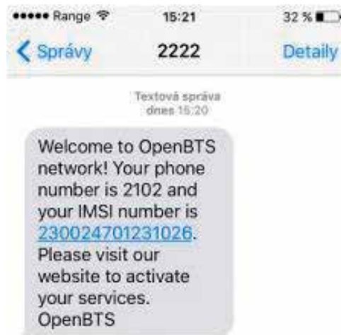
Figure 4. Automatic IMSI registration in OpenBTS network.
