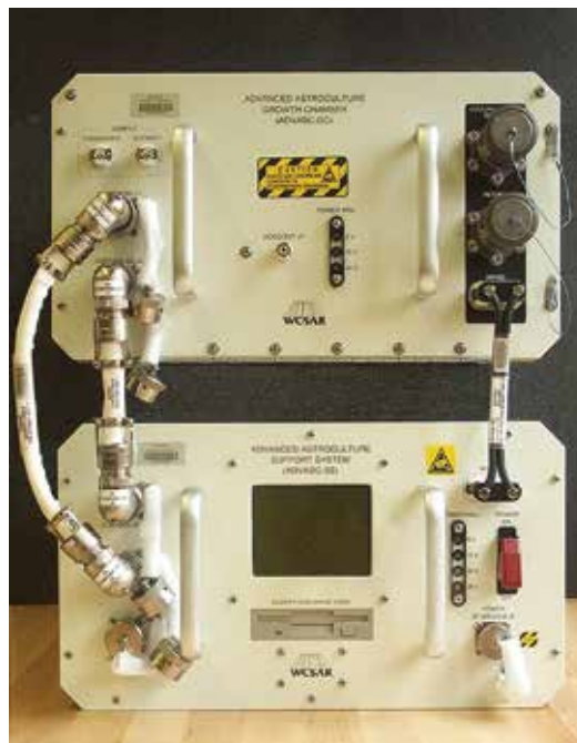
Figure 1. Advanced Astroculture (ADVASC) environmentally controlled plant growth chamber, designed for experiments on the ISS, able to support plant research for a maximum of 6 months in microgravity environment.
