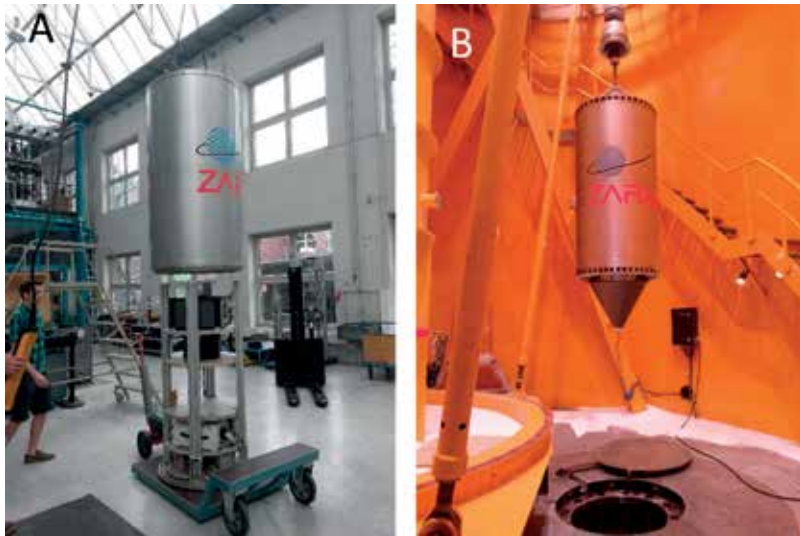
Figure 6. A: Sealing process of the capsule with the aluminium sheath for pressurisation. B: Sealed capsule in the drop tower.
