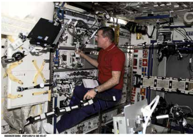
Figure 3. Expedite the Processing of Experiments to the Space Station (EXPRESS) rack 1 on the ISS is pictured on-orbit May 14, 2001, with astronaut James Voss checking ADVASC functioning. Image credit: NASA/JSC. The EXPRESS rack is a multipurpose rack system that houses and supports research aboard the space station.
