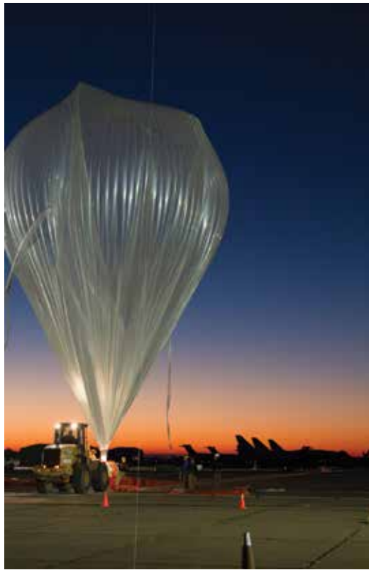
Figure 5. The balloon used for the StratEx mission being filled just as dawn breaks. The restraining fabric can be seen tied near the bottom, restricting the fill of the lower part of the balloon.
