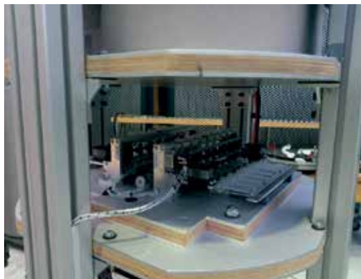
Figure 5. Hydraulic-driven syringes controlled by the capsule control system for fixation experiments with zooplankton.
