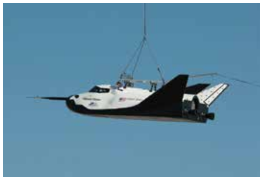
Figure 9. Dream Chaser spacecraft being lifted by an Erickson Air-Crane helicopter during a captive-carry flight test.
