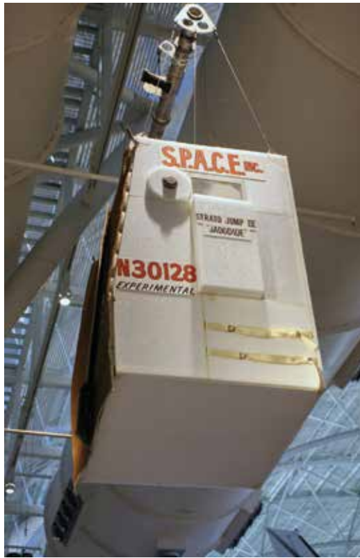
Figure 2. Styrofoam-insulated gondola used by Nick Piantanida during the Strato Jump III mission. Now on exhibit at Smithsonian Institution’s National Air and Space Museum.
