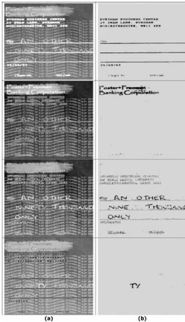
Figure 11. Results of the combined use of automatic segmentation and target visualization of similarity to the main spectra. (a) Visualization of similarity to the spectra obtained by automatic segmentation; (b) the images edited by selecting the brightness range.
