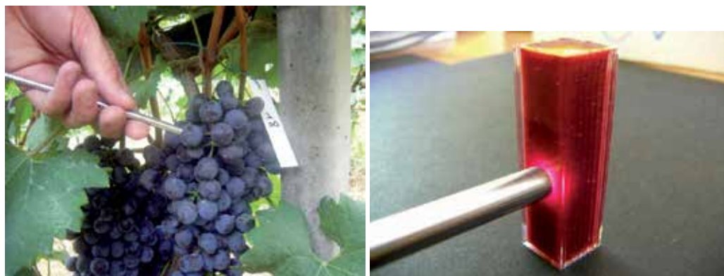
Fig. 9. Images of spectral acquisition phases on fresh berries and on homogenized samples.
