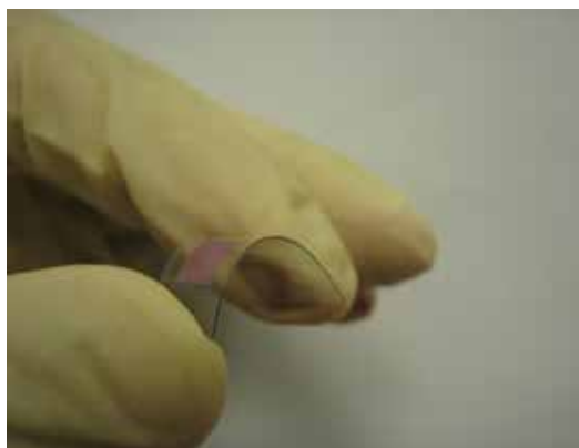
Figure 5. A flexible photoanode with dye-sensitized \text{TiO}_2 film on ITO-PEN substrate.
