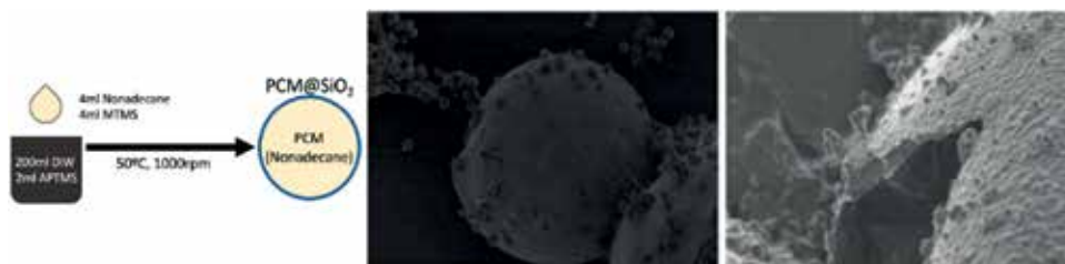
Figure 14. (Left) Illustration of the design of silica-coated nonadecane using MTMS in water medium by Jin et al. (Right) SEM images of PCM microencapsulated spherical capsules: (a) an intact microcapsule and (b) a broken microcapsule of core-shell microstructure [28].
