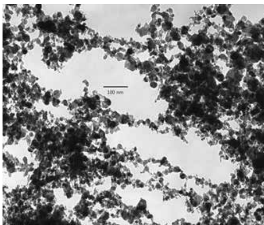
Figure 16. TEM image of NiO nanopowder.
