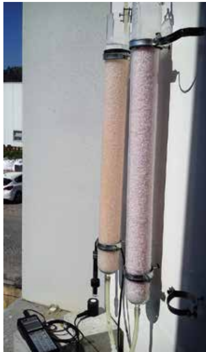
Figure 3. Filtration columns with a quartz porous media for OTC photo-oxidation.
