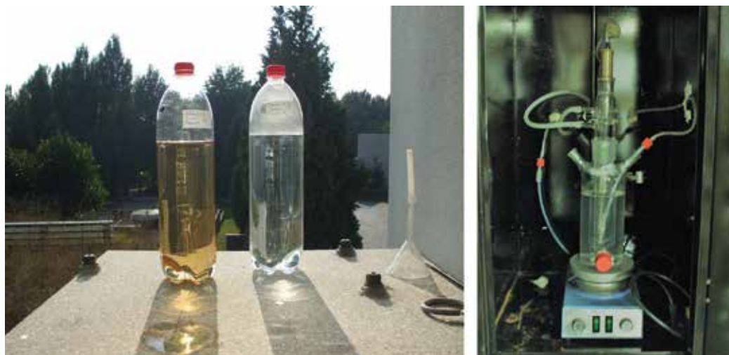
Figure 2. UV radiation sources used in OTC degradation experiments: solar (polyester bottles); UV reactor Heraeus Noblelight .
