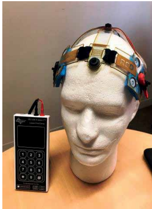
Figure 3. Example of transcranial direct current stimulator (tDCS) setup; mini-clinical trials (mini-CT) Unit, Soterix Medical ® .
