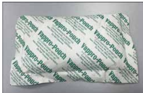
Figure 5. Breathable pouches containing vapor corrosion inhibitor.
