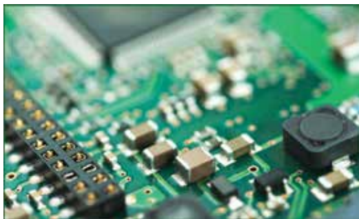
Figure 7. Printed circuit board protected by VCI electrocoat.
