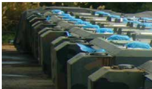
Figure 6. Steel combustible tanks, ready for covering with a VCI protective cloth.
