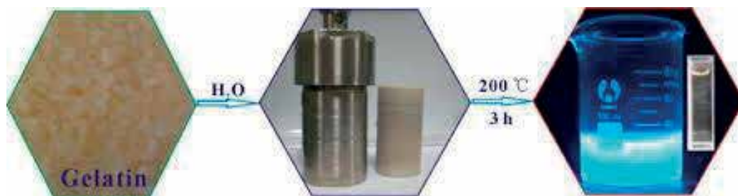
Figure 6. Synthesis of blue emissive carbon quantum dots from gelatin via hydrothermal carbonization process (reproduced with permission from [7]).
