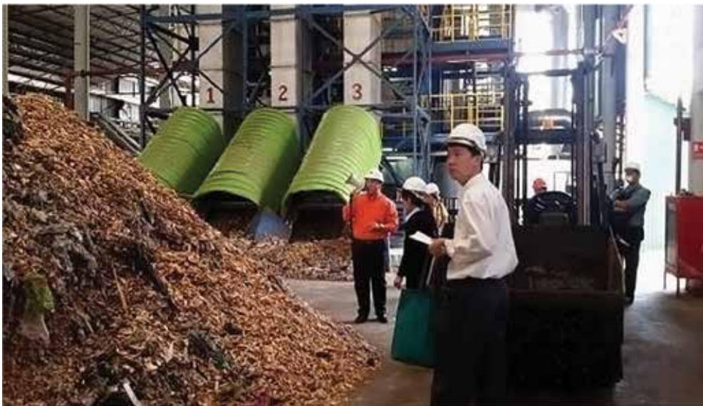
Figure 8. Wood chip mixed with residual waste before gasification.
