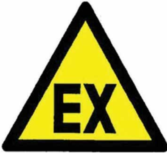
Figure 1. Sign (zone where potentially explosive atmospheres can occur).
