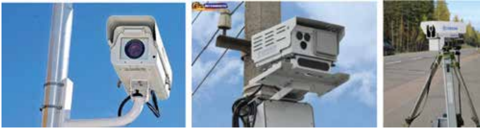
Figure 1. CCTV cameras and photoradar vehicle detector complexes.
