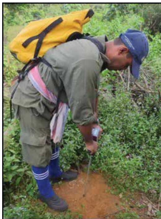
Figure 4. Measuring of soil compaction through penetrometer.
