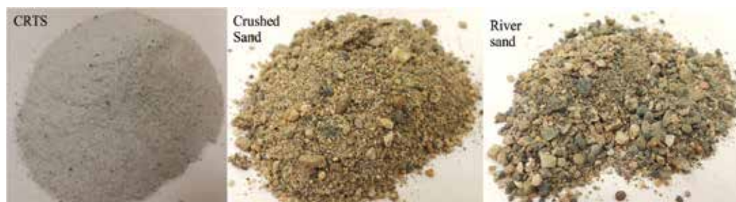
Figure 1. Photographs of CRTS, crushed sand, and river sand used in the study.
