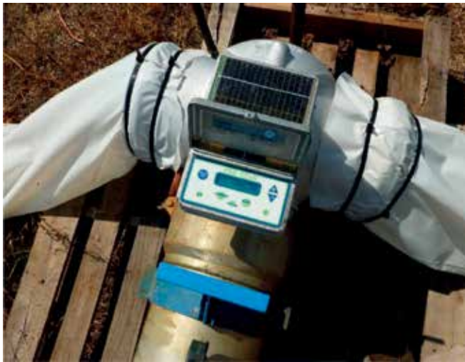
Figure 3. Surge valve used to improve distribution of furrow irrigation in fields.
