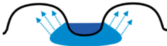
Figure 1. Irrigation water infiltrates into soil below the furrow and wicks to each side and up into beds by capillary rise against gravity through small soil pores.
