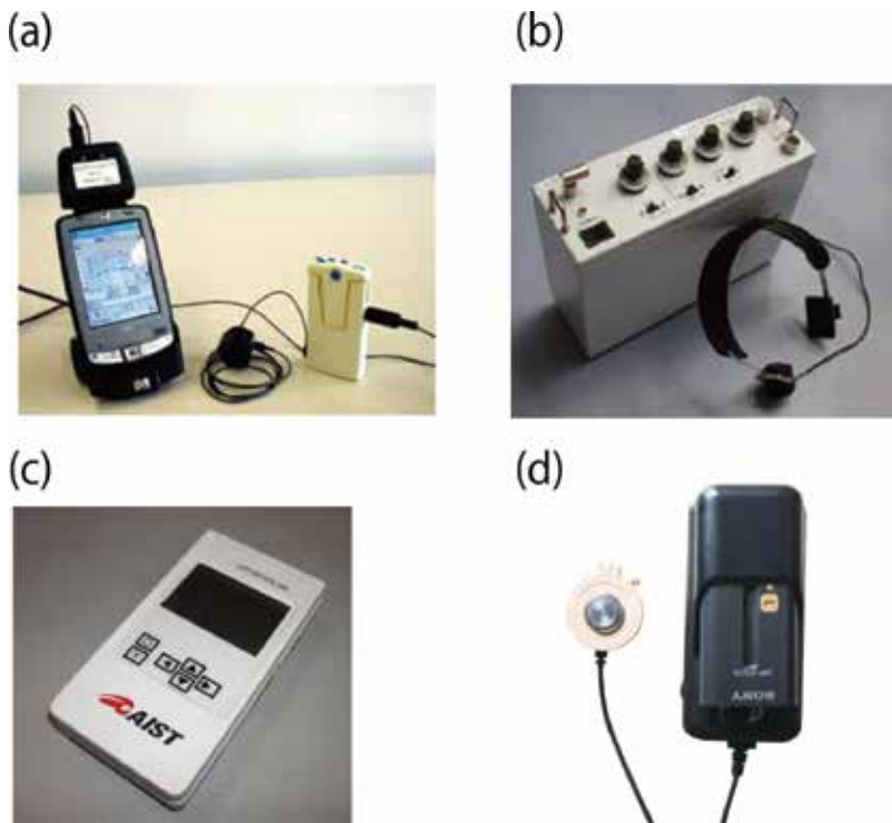
Figure 10. Bone-conducted hearing aids: (a) HD-GU, (b) AIST-BCUHA-003, (c) AIST-BCHA-005, and (d) HiSonic.
