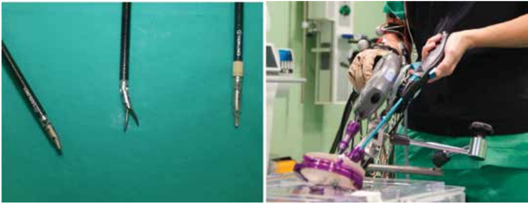
Figure 4. Interchangeable instruments (needle holder, dissector, and scissors) of the Kymerax ® system. Use of the robotic device during LESS training tasks on a box trainer.
