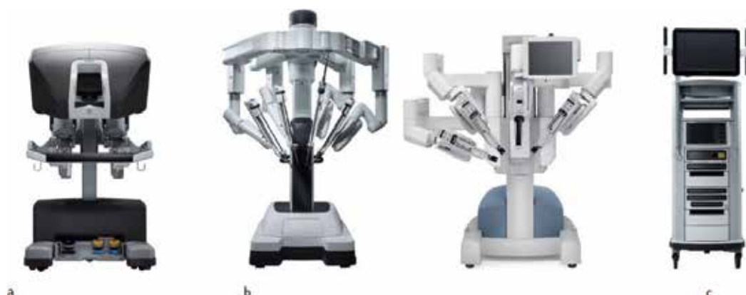
Figure 1. (a) Surgeons console; (b) patients side-cart; and (c) vision tower.
