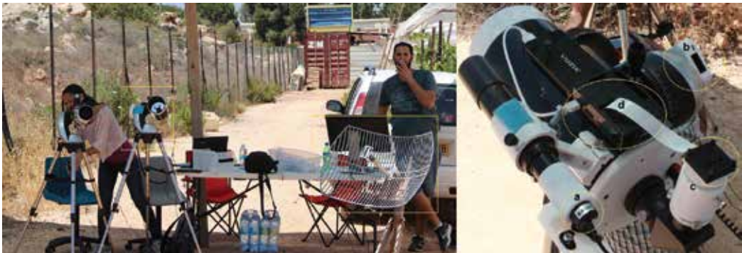
Figure 11. HAB ground station (GS): Left: The GS in general: two robotic telescopes with (auto-track) and a high gain 24dBi Wi-Fi antenna. Right: the robotic telescope: (a) A view-finder webcam. (b) A Wi-Fi + 3G router. So the telescope can be controlled globally. (c) A Pi-camera mounted to the telescope eye-view. (d) A Raspberry Pi which controls the telescope using either visual tracking and GPS coordinates.
