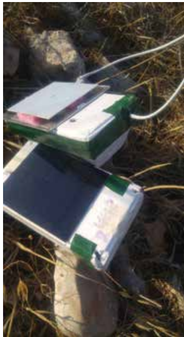
Figure 4. The retrieved payloads from the above experiment were found on a distant field, about 100 km from the point of launch. The crashing location was transmitted by the iridium communication system after the crash. In the picture, the upper box is the secondary payload and the main is the lower box.
