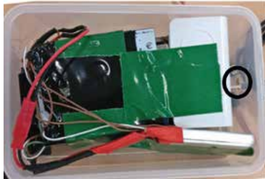
Figure 7. A typical thermal-balanced-payload, notice the ventilation hole marked with a circle.
