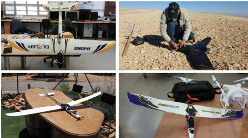
Figure 15. Four different models of RTH micro drones. Each of them was tested for autonomous flight launched from a balloon.
