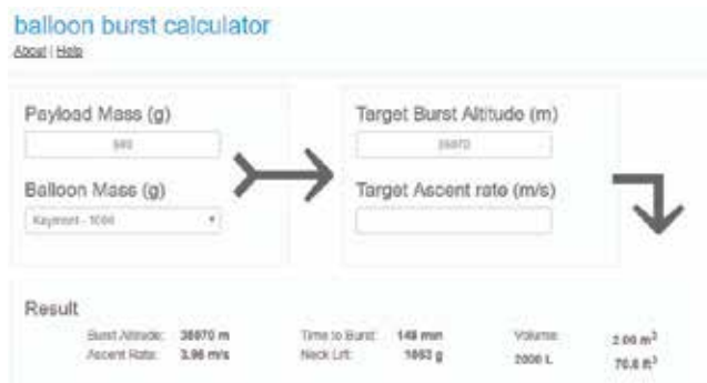
Figure 2. An HAB’s lift and burst calculator, from: http://habhub.org/calc/ .
