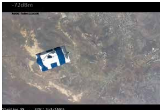
Figure 13. The smartphone payload shot from an upper payload based on a Raspberry-Pi camera equipped with a long-range Wi-Fi transmitter. The picture was taken at about 9.7 km above ground.
