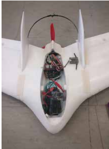
Figure 19. 290 g RTH micro-UAV, with a release carbon strip on its backend.
