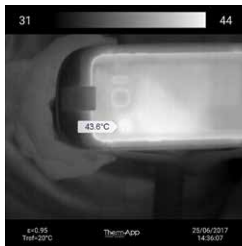
Figure 6. Thermal analysis of an android phone using a thermal camera (Op-gal’s Therm-app).
