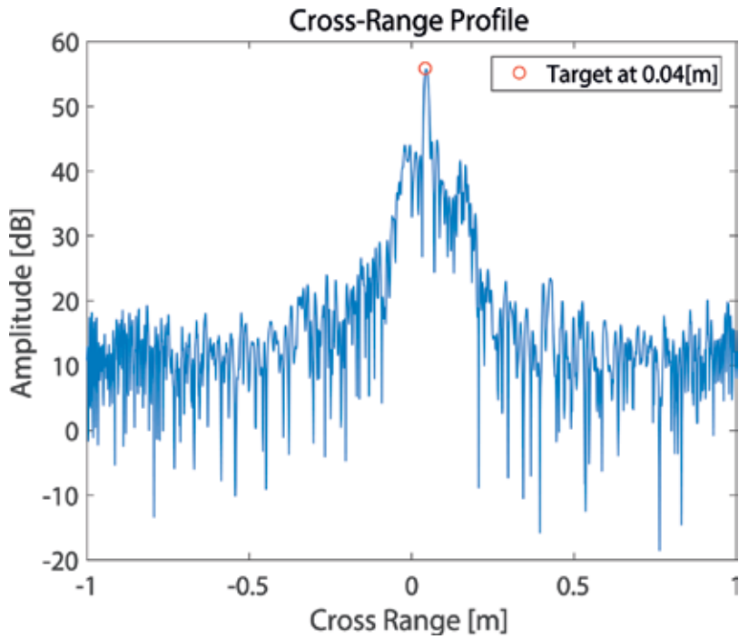
Figure 34. Cross-range profile of the impulse target with motion compensation.
